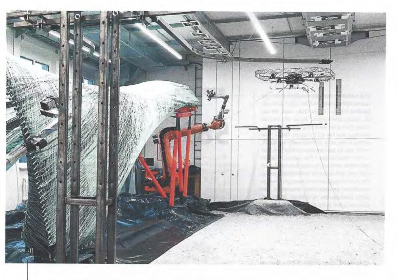
Fabrication of a pavilion made from carbon fiber-reinforced composites is underway, using fiber-winding robotic arms and an autonomous drone "weaver." For this commission for the University of Stuttgart's Institute for Computer-Based Design, SGL Group was tasked with delivering 104 kms of SIGRAFIL® 50k carbon fiber. The design technology was modeled on the larvae of the apple leaf moth, which spins its cocoon on apple tree leaves using long threads.
